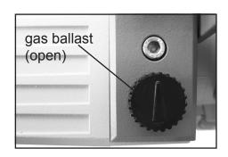
For **condensable vapors** (water vapor, solvents, etc.):
