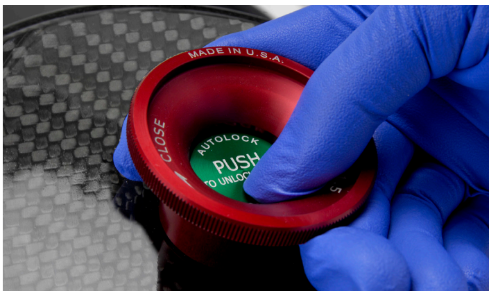
Figure 2-10: Pressing the Auto-Lock key
