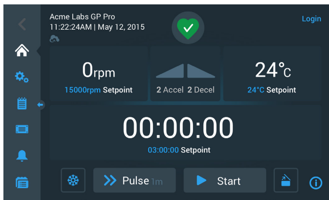
Figure 3-3: Touchscreen Display for Refrigerated Centrifuge
