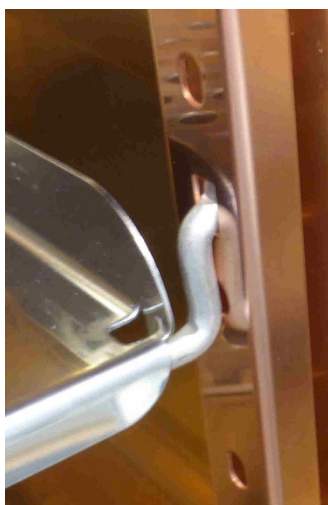
Figure: Perforated Shelf Installation
