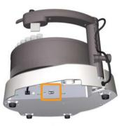
Make sure that all unused UniNet-9 ports on the ÄKTA pure instrument are 4 plugged with jumpers.
