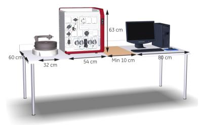
**Note:** Fraction collector F9-R requires 10 cm free space above the fractionation arm for handling of tubes.
