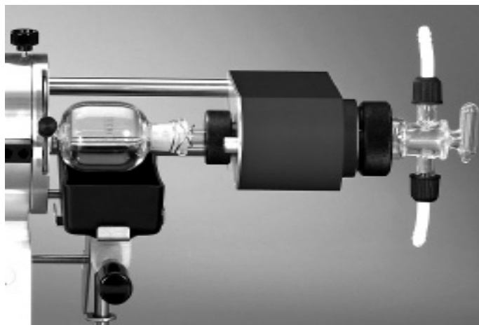
Fig. 2: Ball tube drive complete
