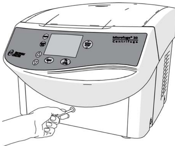
Figure 3.3 Manually releasing the door lock with the Allen wrench
