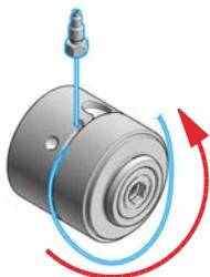
**12** Insert the fixing screw, so that the capillary cannot leave the groove.
