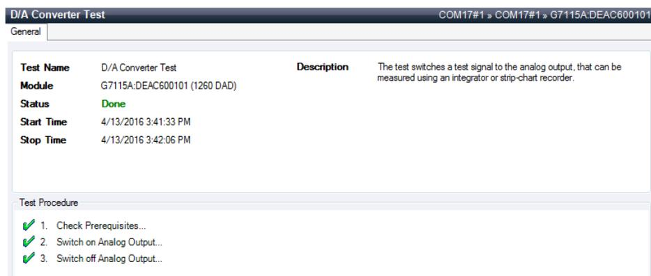
Figure 41 D/A Converter (DAC) Test – Results
