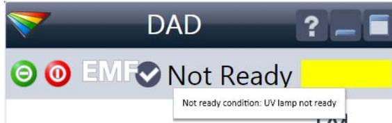
Module Status shows Run / Ready / Error state and "Not Ready text" or "Error text"
