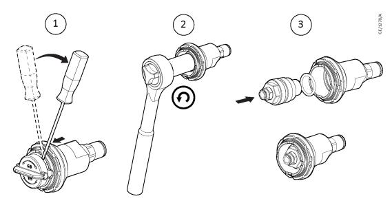
The manually operated gas ballast knob can be replaced by a gas ballast adaptor which enables external electrically actuated valves or a controlled gas supply to be used through a 1/4 inch push fit connector. To install the gas ballast adaptor:
